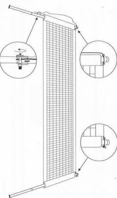
Step 5: Fasten the carabiner on the guide rope and the eyebolt set on the aluminum pole, and nail the guide rope to fix the erected aluminum poles. the two ground nails is 3 to 4 feet. Then, erect the aluminum poles, keep them vertical, adjust the needle on the guide rope to the ground, to make that the distance between the single guide rope and
