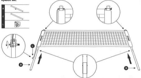
Step 5: Fasten the carabiner on the guide rope and the eyebolt set on the aluminum pole, and nail the needle on the guide rope to the ground, to make that the distance between the single guide rope and the two ground nails is 3 to 4 feet. Then, erect the aluminum poles, keep them vertical, adjust the guide rope and plastic fork to fix the erected aluminum poles.
