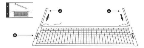
Step 4: Connect the upper and bottom parts of the aluminum pole, and pass one end of the pole on the net side through the eyebolt set, and connect it to the tension adjuster. The other end is attached to the eyebolt set.
